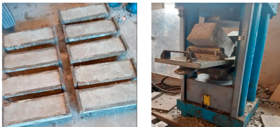
Fig. 6. Concrete flexural strength test.
