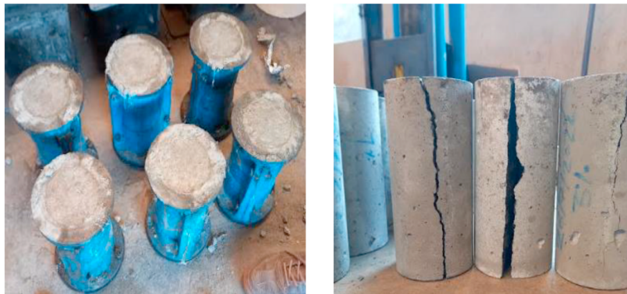
Fig. 5. Concrete splitting tensile strength test.
