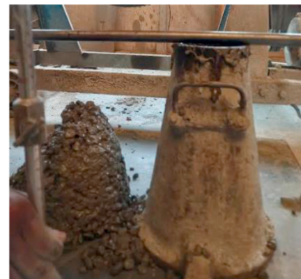
Fig. 3. Concrete workability test.
