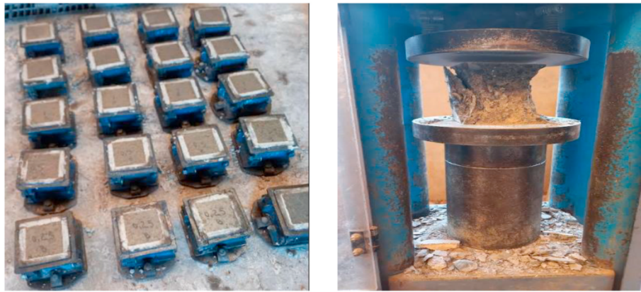
Fig. 4. Concrete compressive strength test.
