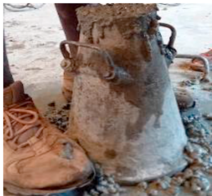
Fig. 3. Concrete workability test.
