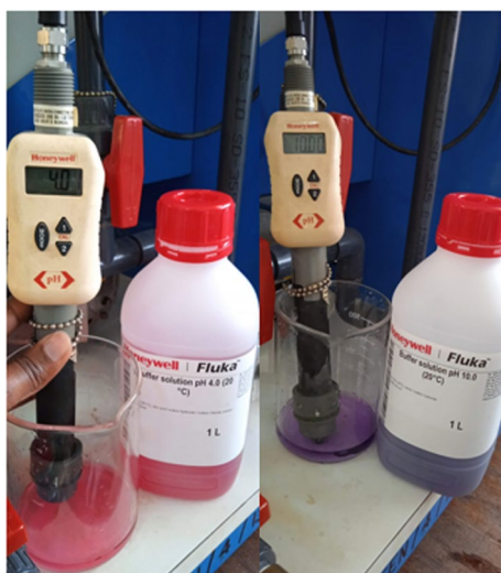
Fig. 2 Chemical solutions used (pH 4.0 and pH 10.0)
