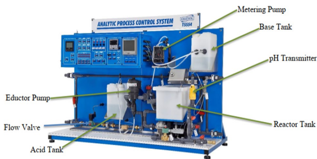
Fig. 6 Amatrol Analytic process control system
