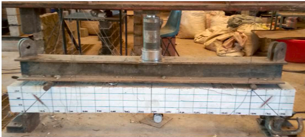
Fig. 7. Shear and flexural beams test setup and instrumentation.
