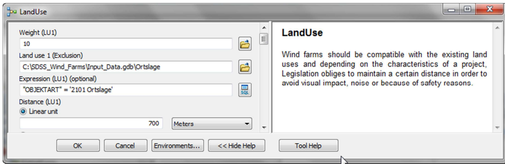
Figure 3 Dialog box for a Land Use in ModelBuilder. This image represents the dialog box which appears when running the submodel of Land Use for models 2 or 3 from ModelBuilder.
