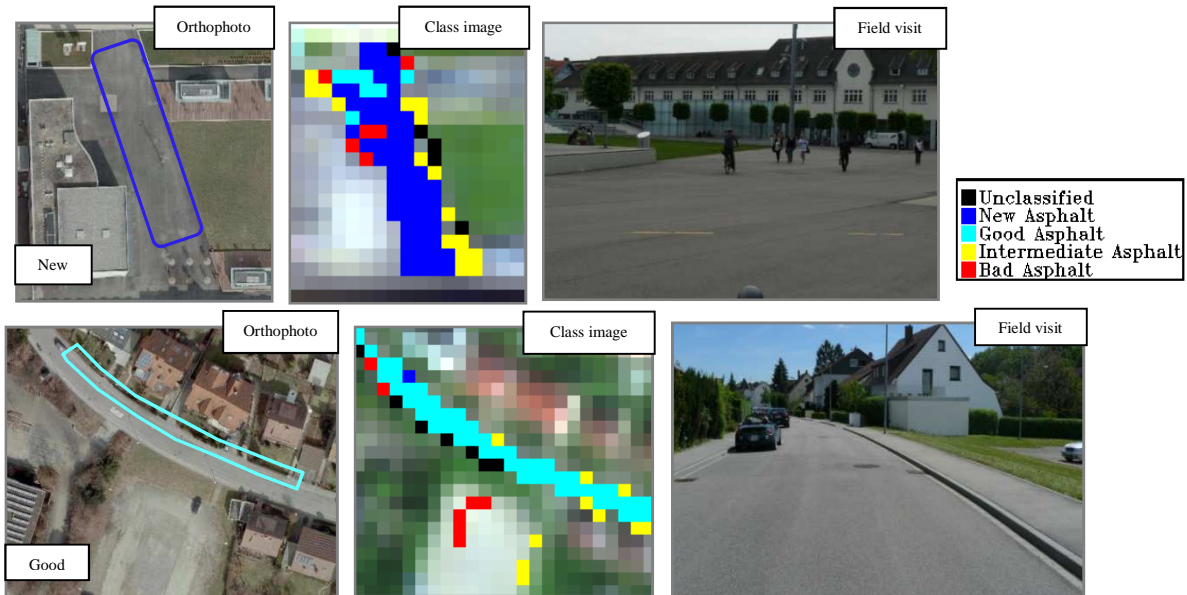
Figure 5: New (upper) and good (lower) asphalt condition classification.
