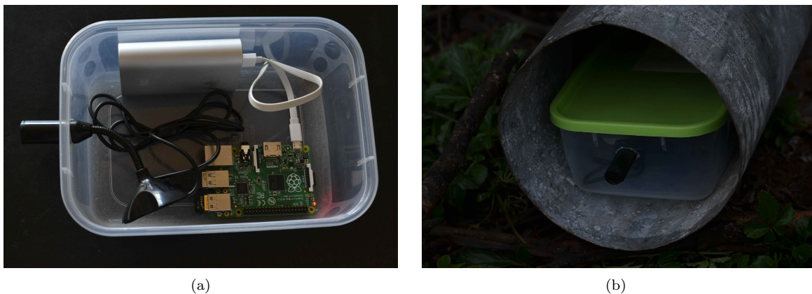
Figure 1. The Raspberry Pi based acoustic sensor system (a) and the system deployed at the DeKUT conservancy (b).
