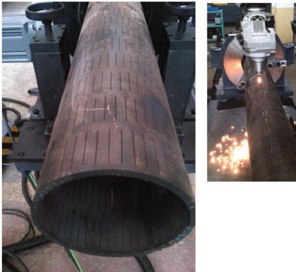
Figure 5 A slotted steel pipe used in the oil industry for heavy oil production; the slots are created by laser cutting (Rath and Gaebler, 2017).
