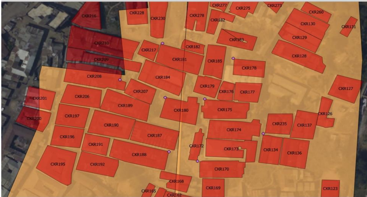
Figure 7. Digitized structures as they appear on the STDM system, the GPS points that guided digitization and structure numbers are displayed
