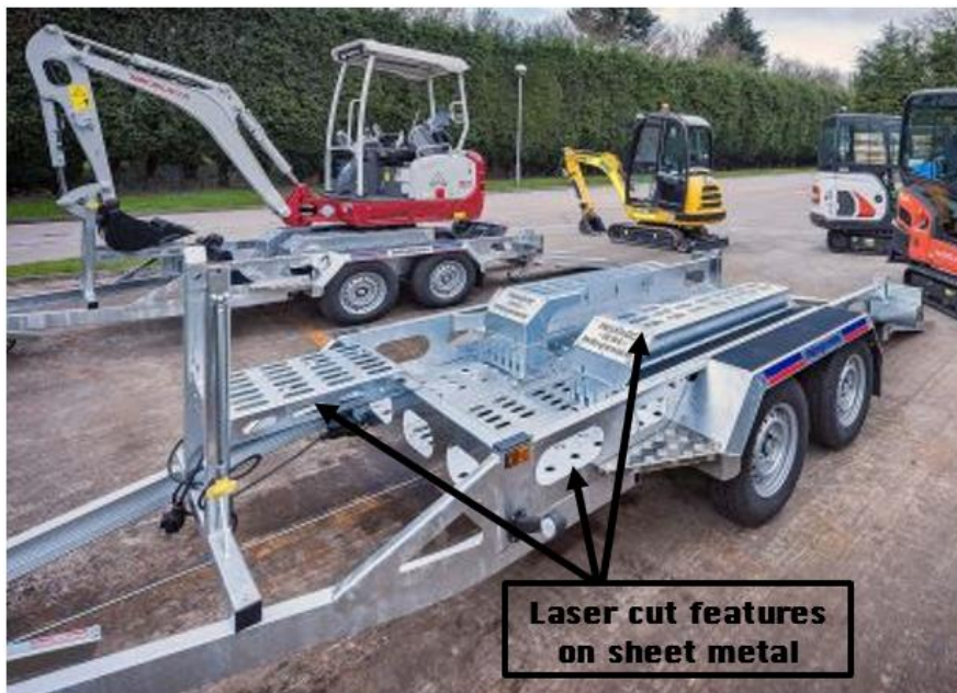
Figure 3 Trailer body with sheet metal component parts having laser-cut holes and slots (Larcombe, 2017).
