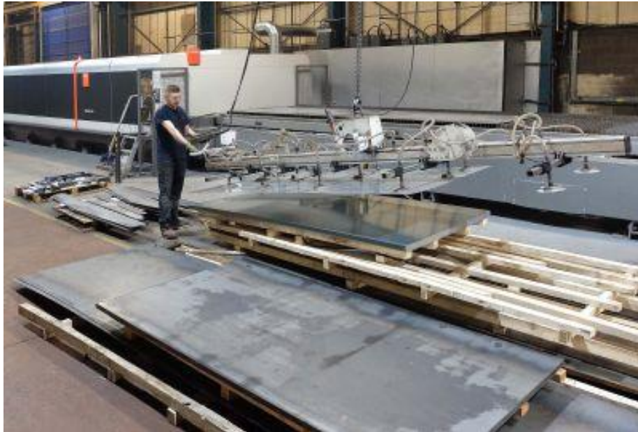
Figure 4 A suction-pad lifting system for manually transferring sheet metal on and off the laser cutting shuttle table (Larcombe, 2017).
