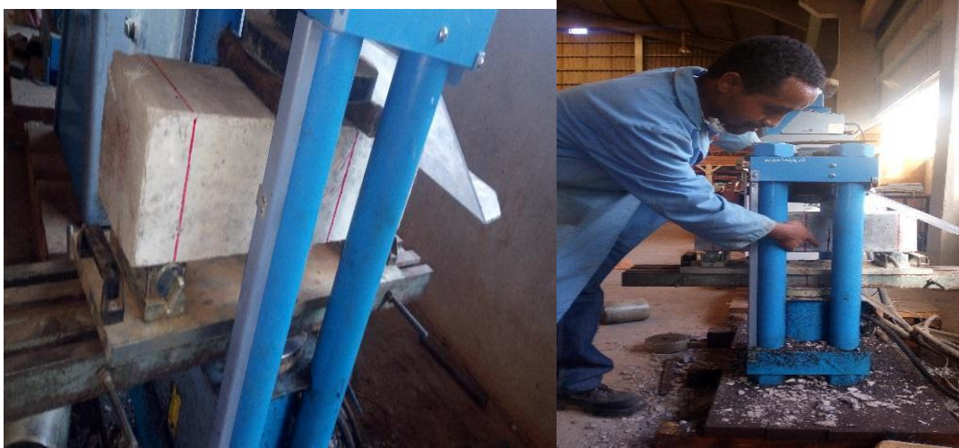
Figure 1 Compressive Strength test in laboratory Figure 2 Tensile Splitting strength test in laboratory
