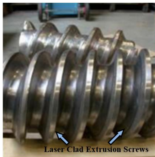
Figure 7. Laser cladding of pet-food granulate extrusion screws extends screw lifetime (Laser Cladding Venture (LCV), 2017)
