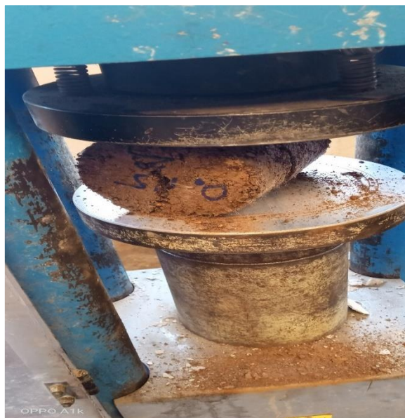
Figure 6: Splitting tensile test
