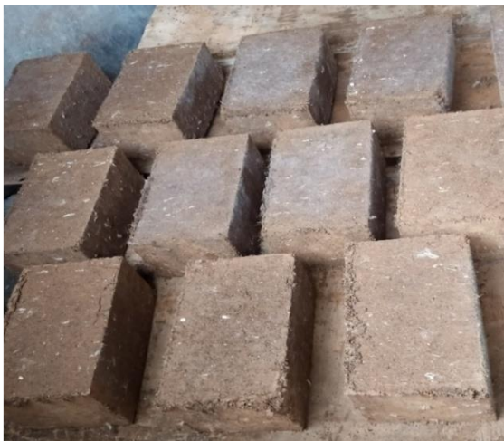
Figure 5: Bricks under curing
