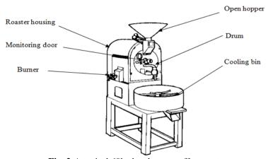
Fig. 2:A typical 60kg batch-type coffee roaster
