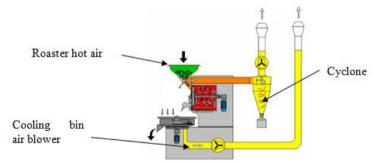
Fig. 5: Ideal conceptual model of an improved coffee roaster
