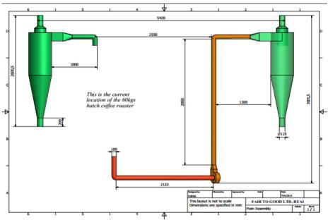
Fig 6:Design alternative for cyclones for the 60kg coffee roaster
