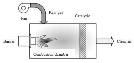
Fig.7: Catalytic oxidation
