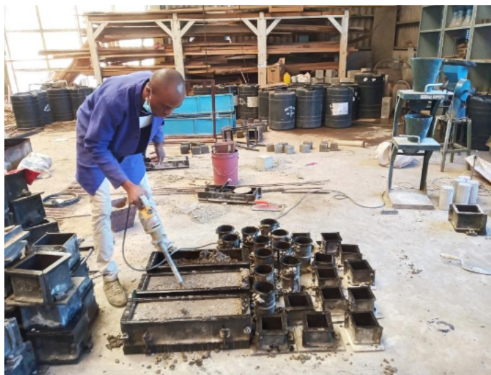
Figure 4. Concrete casting using cubic and cylindrical moulds
