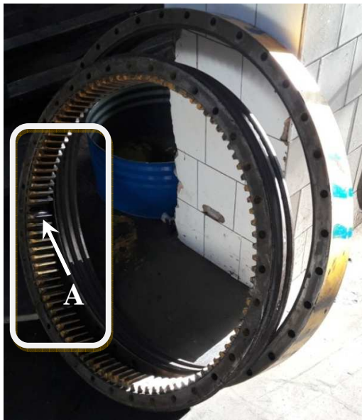
Figure 8. Damaged teeth on a toothed ring of a slewing bearing.
