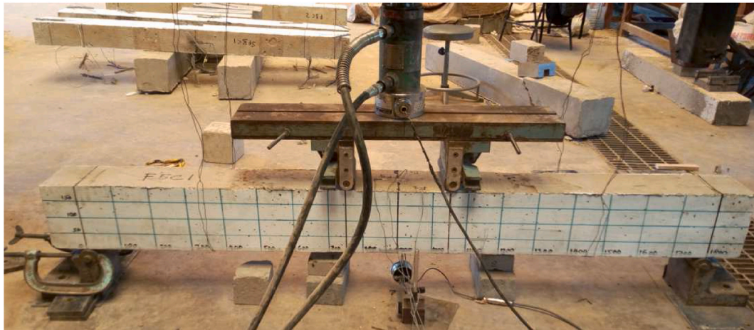
Fig. 5. Flexural beams test setup and instrumentation.
