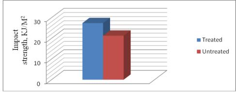
Figure 3: Effect of alkali treatment on the impact strength of the composites
