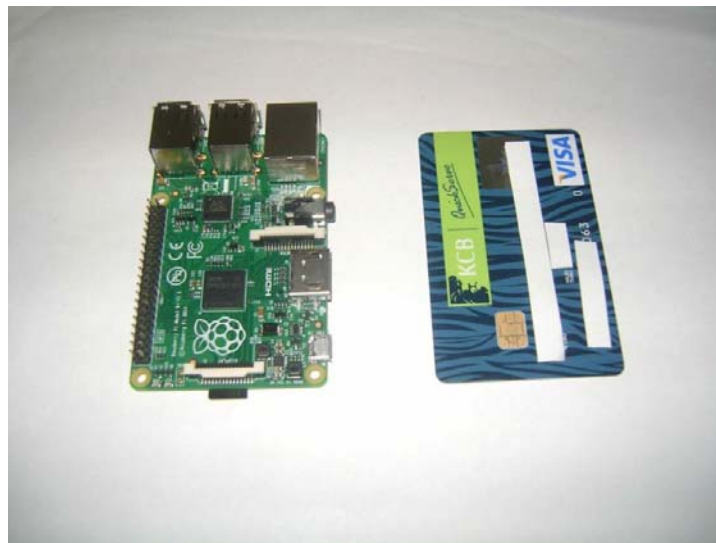
Figure 1: The Raspberry Pi model B+. A Kenyan Bank card is shown for comparison.
