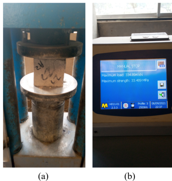
Figure 2.2: (a) Cube under compressive strength test, (b) reading and recording of results
