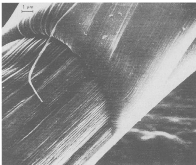
Figure V.4: Scanning electron micrograph of skin peeled polyester fiber. Reproduced by courtesy of H. R. Billica. 34
