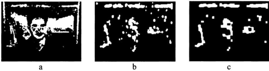
Fig. 8. a) averaged out binary mask, b) multiplied with averaged out wavelet coefficients, c) after morphologic operations with suitable face qualifiers selection.
