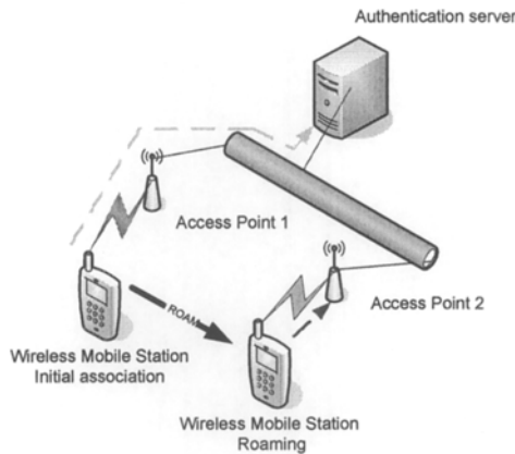
Fig. 4. Association of Wireless Mobile Station to Access Points in roaming process according to 802.11r standard
