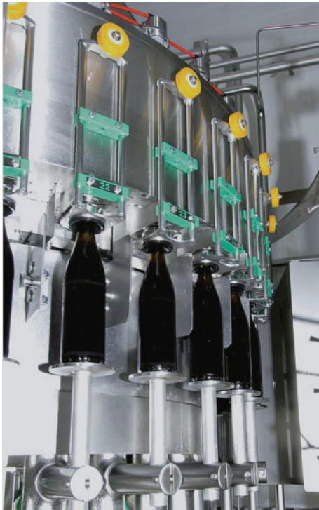
Figure 12.10 Filling with a mechanical filling system.
