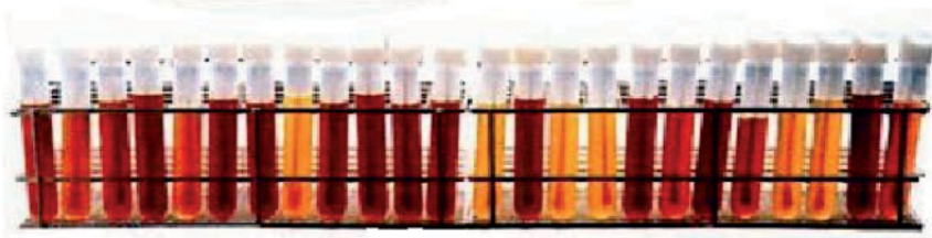
Figure 18.8 Biological situation in the bottle cellar as presented on swab samples. Three days aerobic incubation at 25–28 °C (six of 24 samples with result = 25%).
