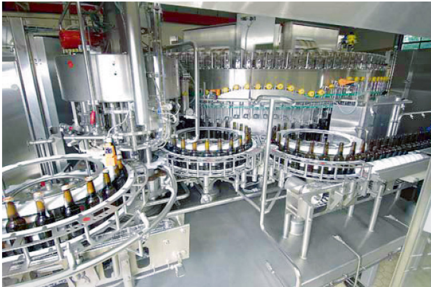
Figure 12.13 Sensometric VPVI with crowner.
