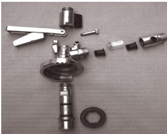
Figure 14.6 Dispensing head on top of a keg.
