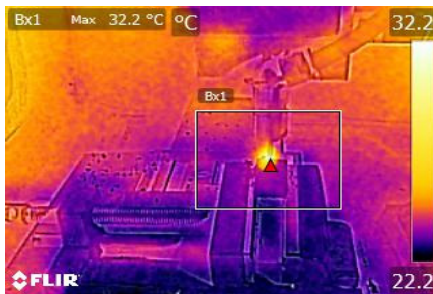
Figure 2. IR image of sample during machining.
