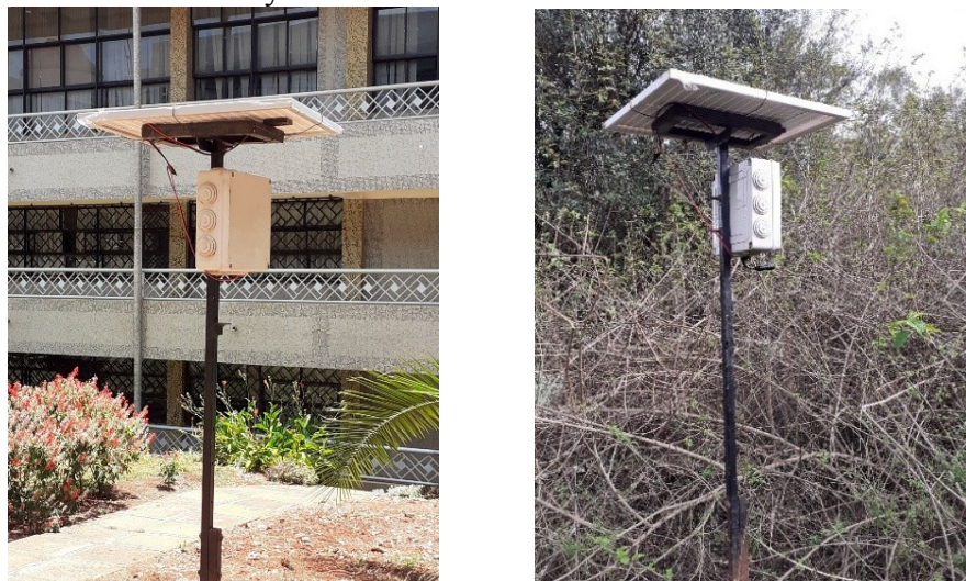
Figure 1: DSAIL Bioacoustics System deployment outside the university Resource Centre for power analysis of the system (left) and at the university conservancy to collect acoustic data of birds (right).
