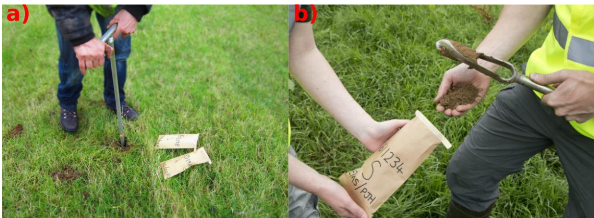
Figure 3.22: Soil sampling using a soil auger: a) soil auger being driven into the ground; b) the soil sample from the ground is placed in a soil bag. Images accessed from http://www.tellus.ie/ on 1/2/2018.
