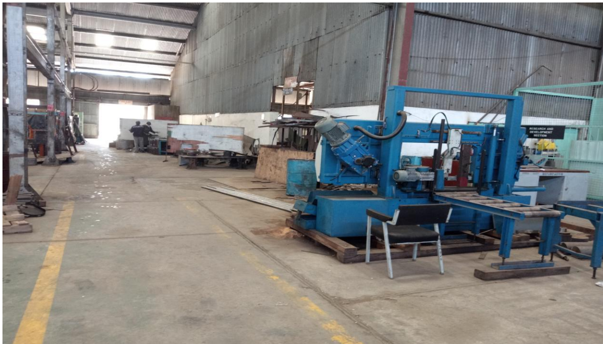
Figure 1.3: Bandsaw and the light fabrication section being located along the gangway in the workshop
