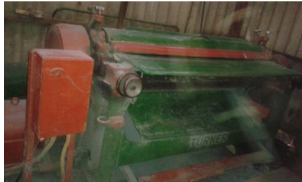
Figure 0.8: Buffing machine. Source: STL
