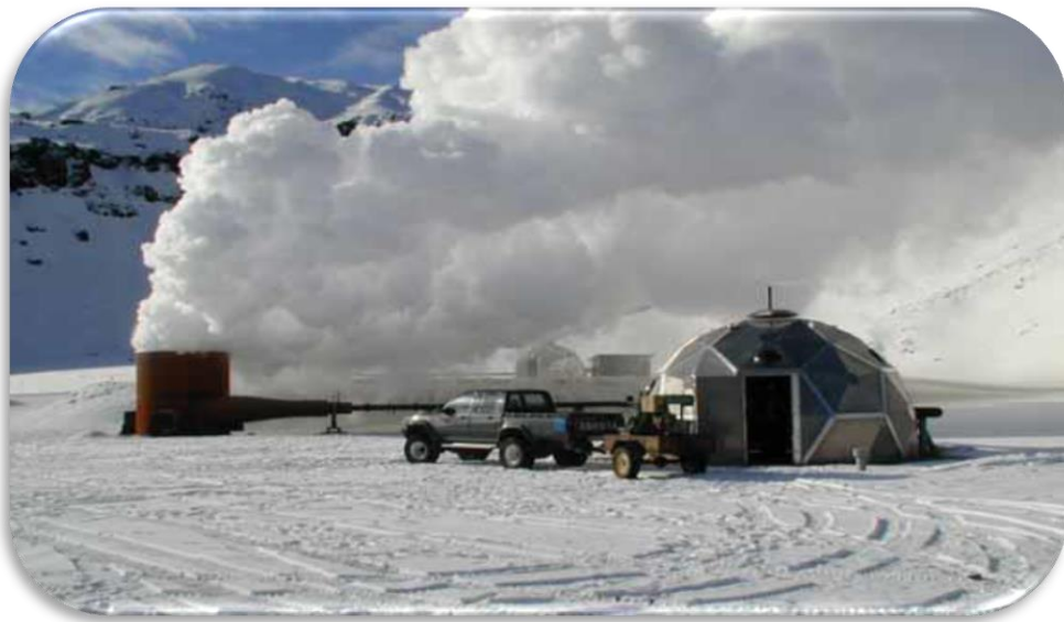
Figure 2. 4: A successful Production well discharging for well testing in Reykjavik, Iceland
