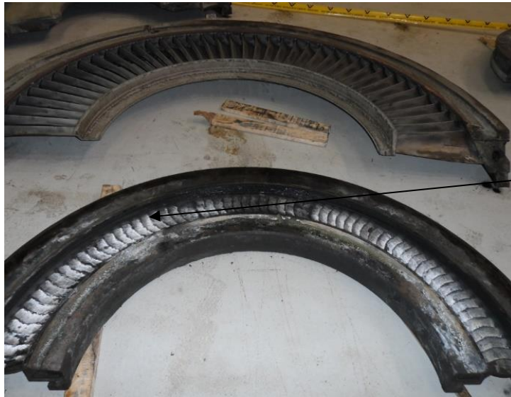
Figure 3. 5: Turbine nozzles with Silica Scales.
