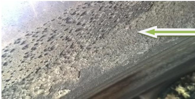
Figure 2. 8: Eroded turbine diaphragms
