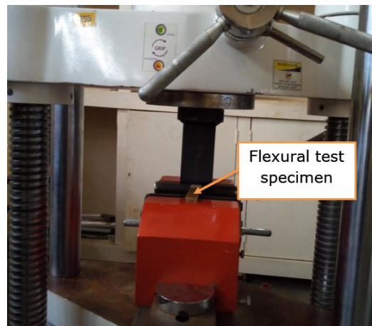
Figure 2.10. Test specimen under flexural loading
