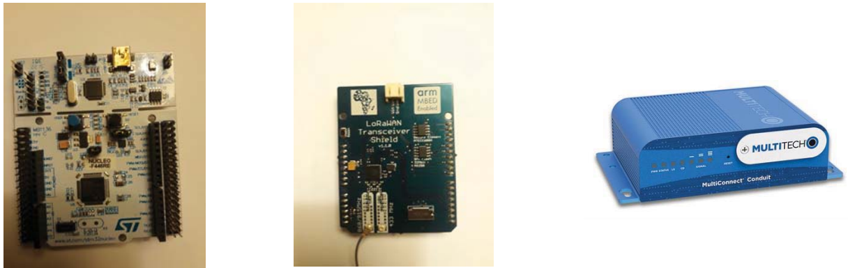
Figure 1: The Nucleo-F446RE development board ( left), custom LoRaWAN transceiver shield (middle) and MultiTech gateway.
