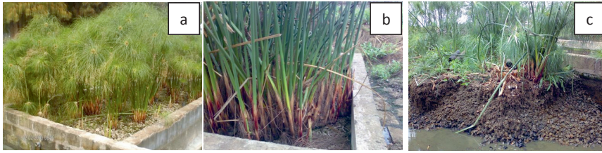
Fig. 3.1: Planted pilot wetland cells showing (a) successful establishment of tropical macrophyte Cyperus papyrus in the pilot gravel beds, (b) progressive increase in plant density, shoot length and stem diameter and (c) root penetration within the gravel bed
