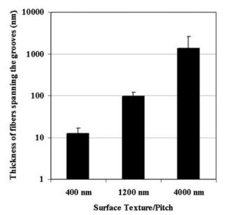
Fig 2. Thickness of the fibers spanning the grooves depends on the groove size. The size of the spanning fibers was obtained from top down SEM measurements. SEM, scanning electron microscopy.
