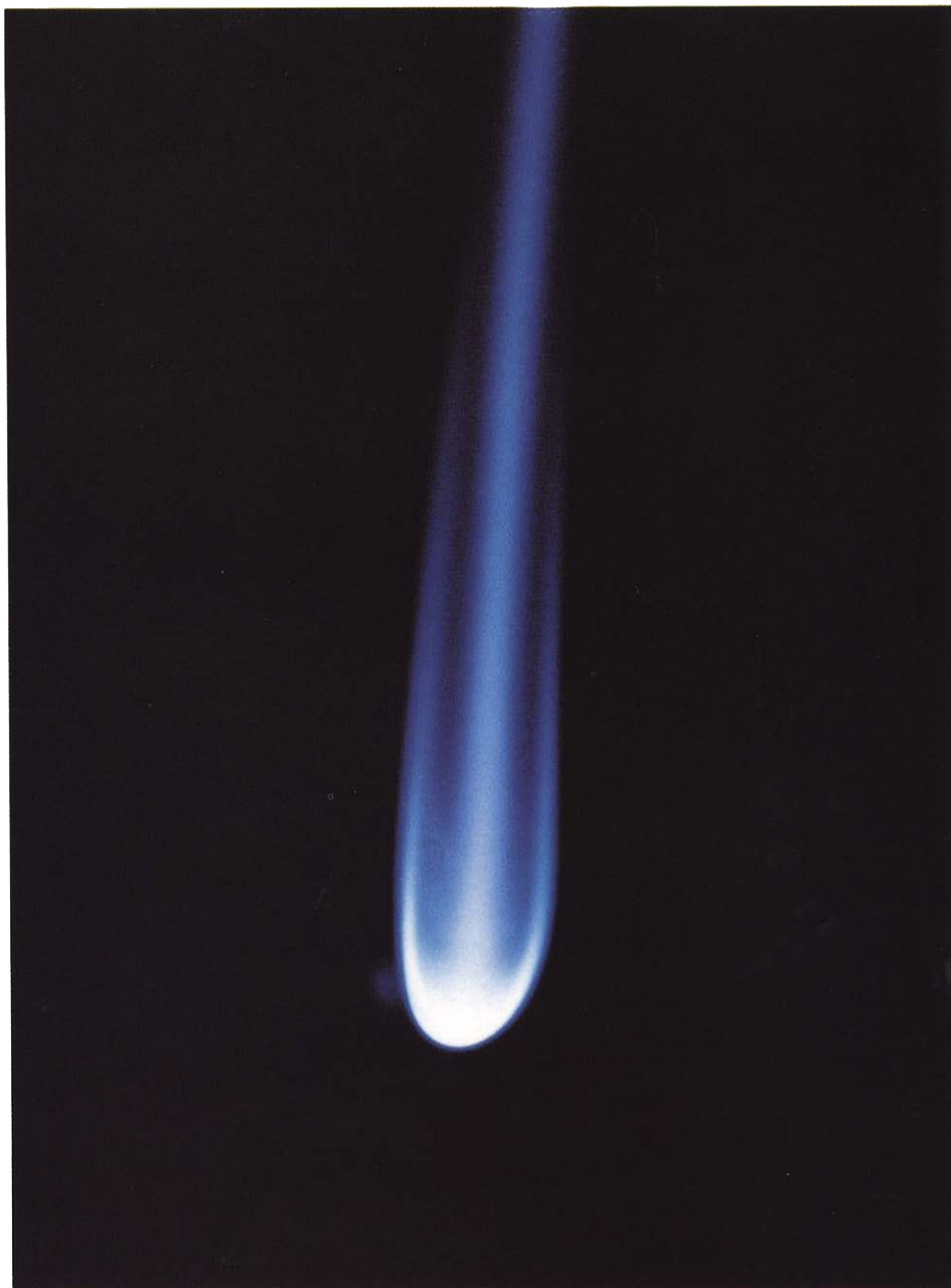
Fig. 1. Typical photograph of a stationary triple flame in a coflowing stream stabilized in the burner described herein. Details can be found in subsections 2.1 and 2.2.
